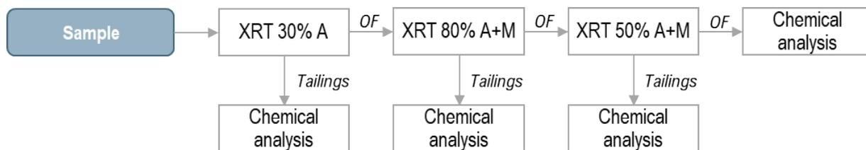
Figure 13-7: Ore Sorter Test Procedure Using XRT Sensor
