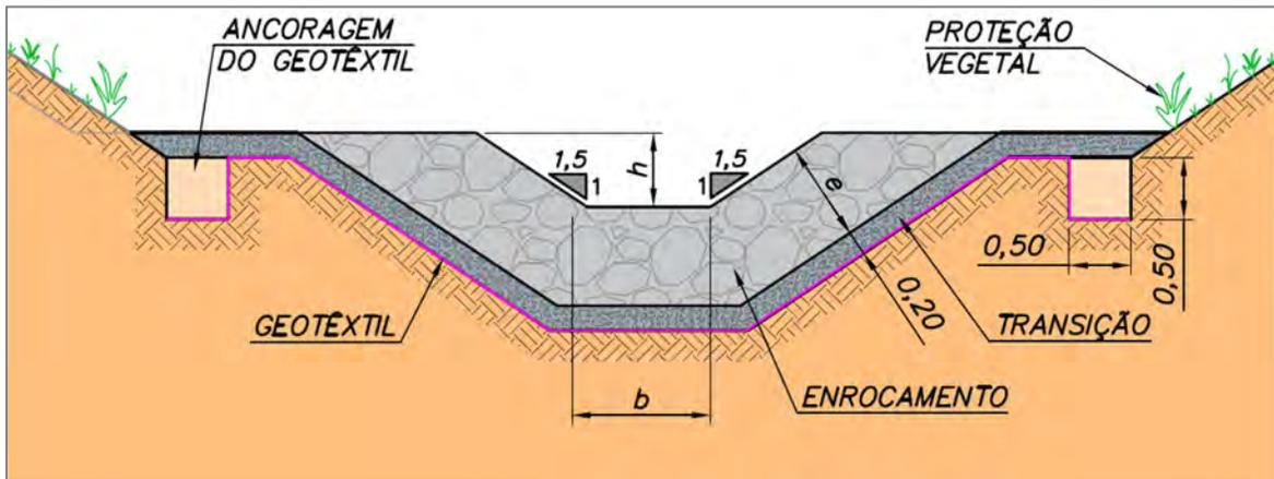
Figure 18-19: Typical Section of Hydraulic Devices Consisting of a Trapezoidal Channel with Rockfill Lining
