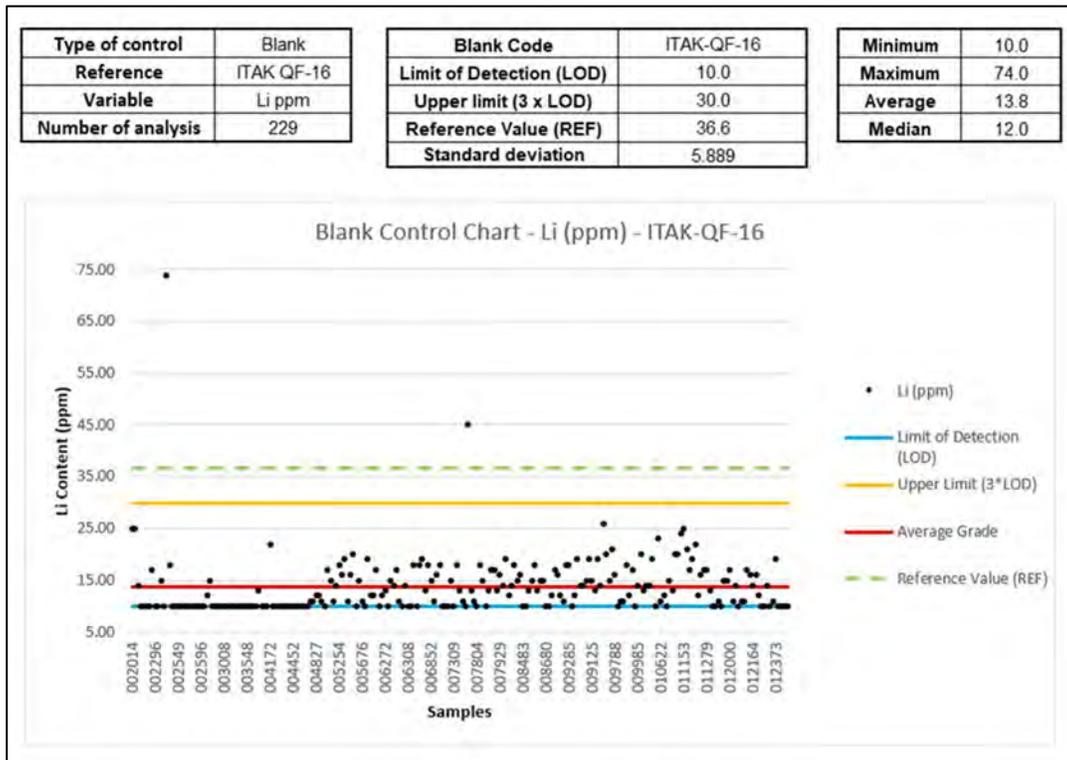
Figure 11-4: Blank Control Chart—ITAK QF-16
