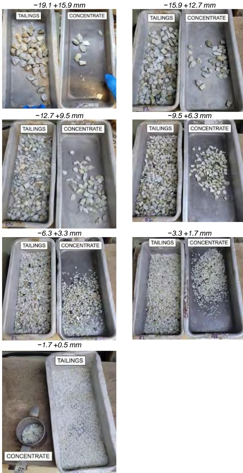
Figure 13-25: HLS Separation for Rougher Stage
