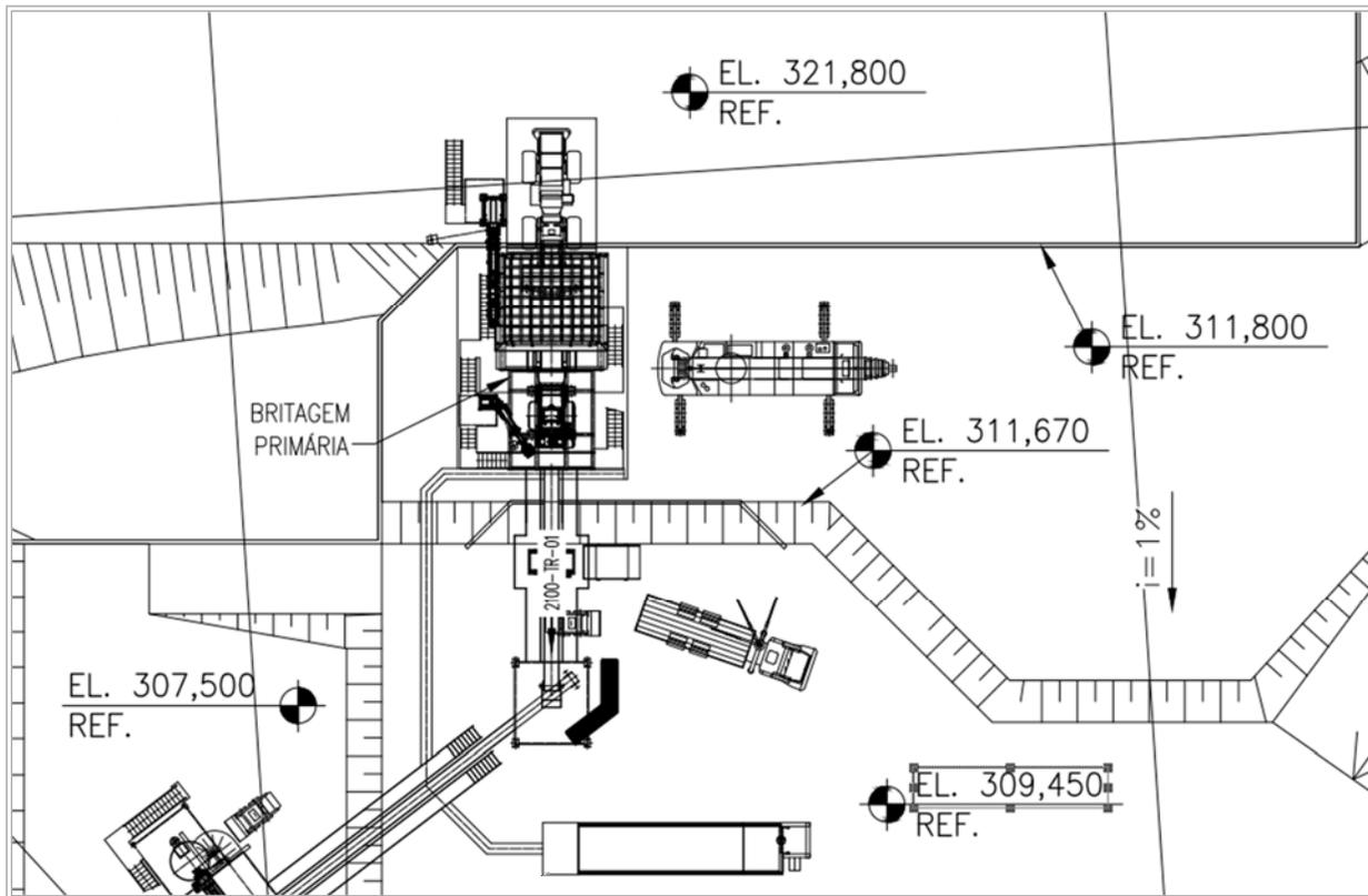
Figure 18-7: Primary Crushing—Crane Patrol and Crane Truck Approach
