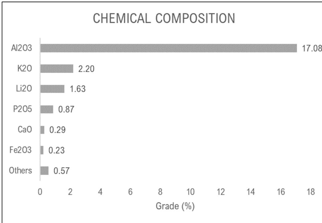
Figure 13-3: Bandaiera Composite Sample Chemical Analysis
