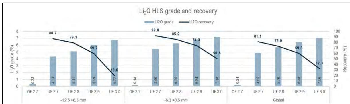
Figure 13-6: Li<sub>2</sub>O Recovery and Grade per HLS Step
