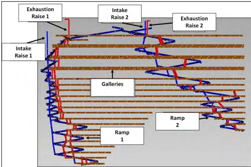
Figure 16-28: Schematic Main Mine Ventilation System
