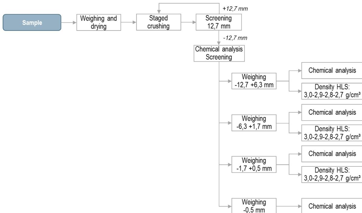
Figure 13-1: Bandeira Composite Sample Preparation Procedure
