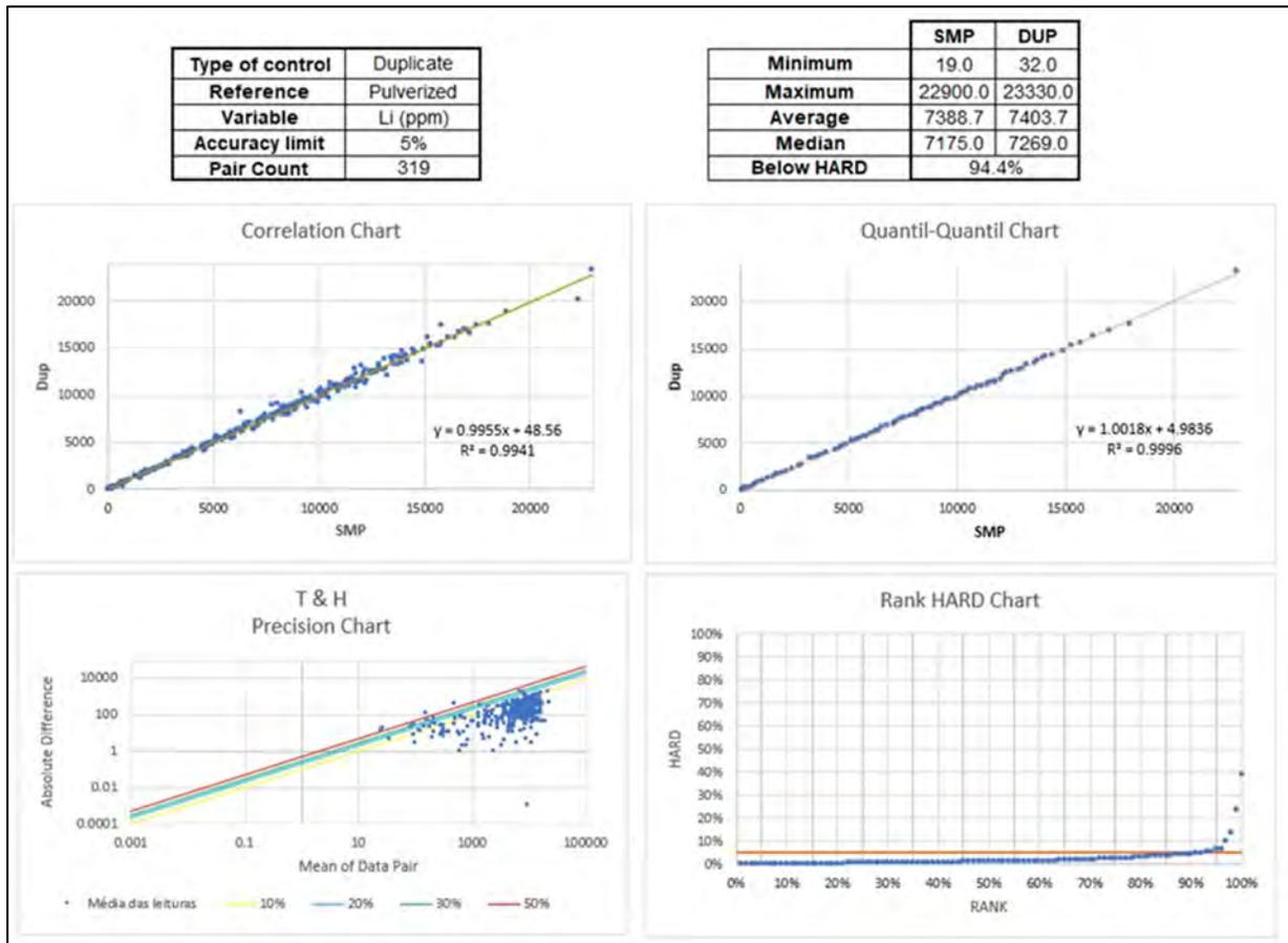
Figure 11-11: Pulverized Duplicates Control Chart
