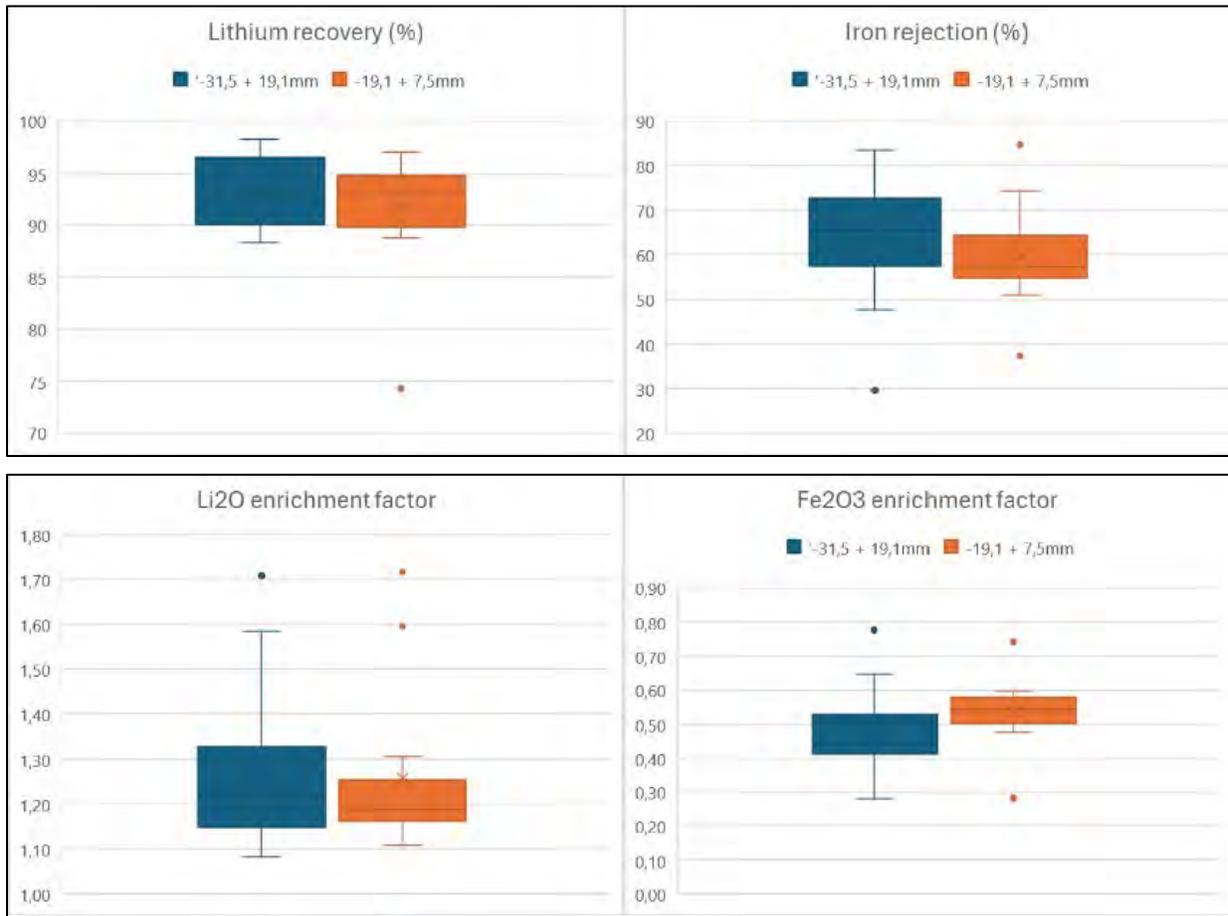
Figure 13-21: Ore Sorter Results for Lithium and Iron
