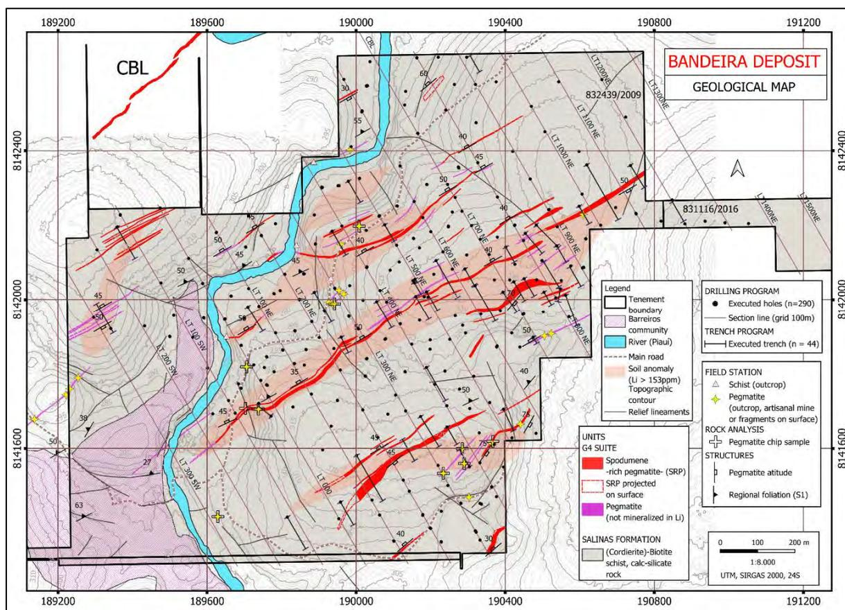
Note: The pegmatite veins are projections of the known intrusions based on the intercepts in drill holes. The attitude of each vein is based on the modelled veins.
