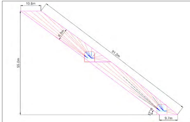
Figure 16-23: Longhole Drilling
