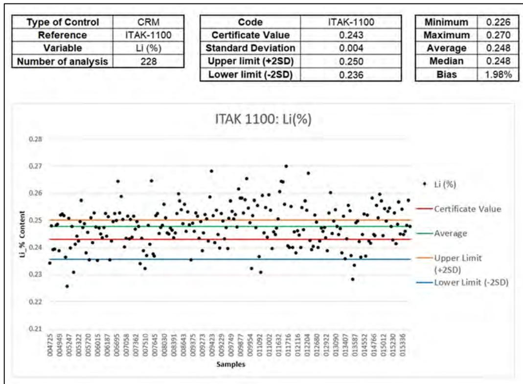
Figure 11-6: Standard Reference Material Chart—ITAK 1100
