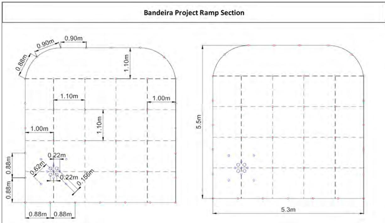
Figure 16-24: Drilling and Blasting Plan for the Ramps
