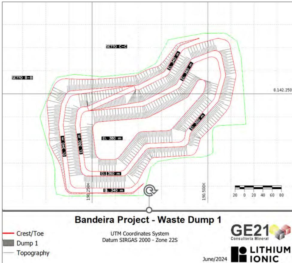
Figure 18-13: Waste Dump 1 Section
