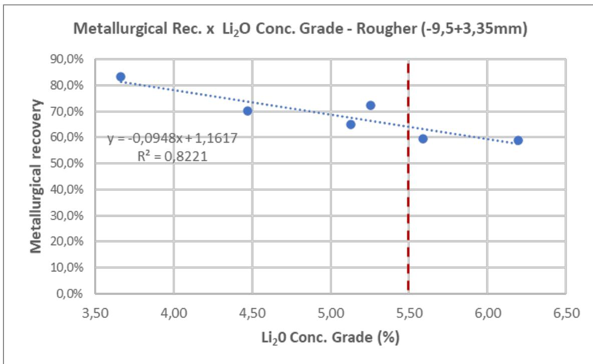
*Figure 13-30: Rougher Coarse Metallurgical Recovery x Li<sub>2</sub>O Grade in Concentrate*
