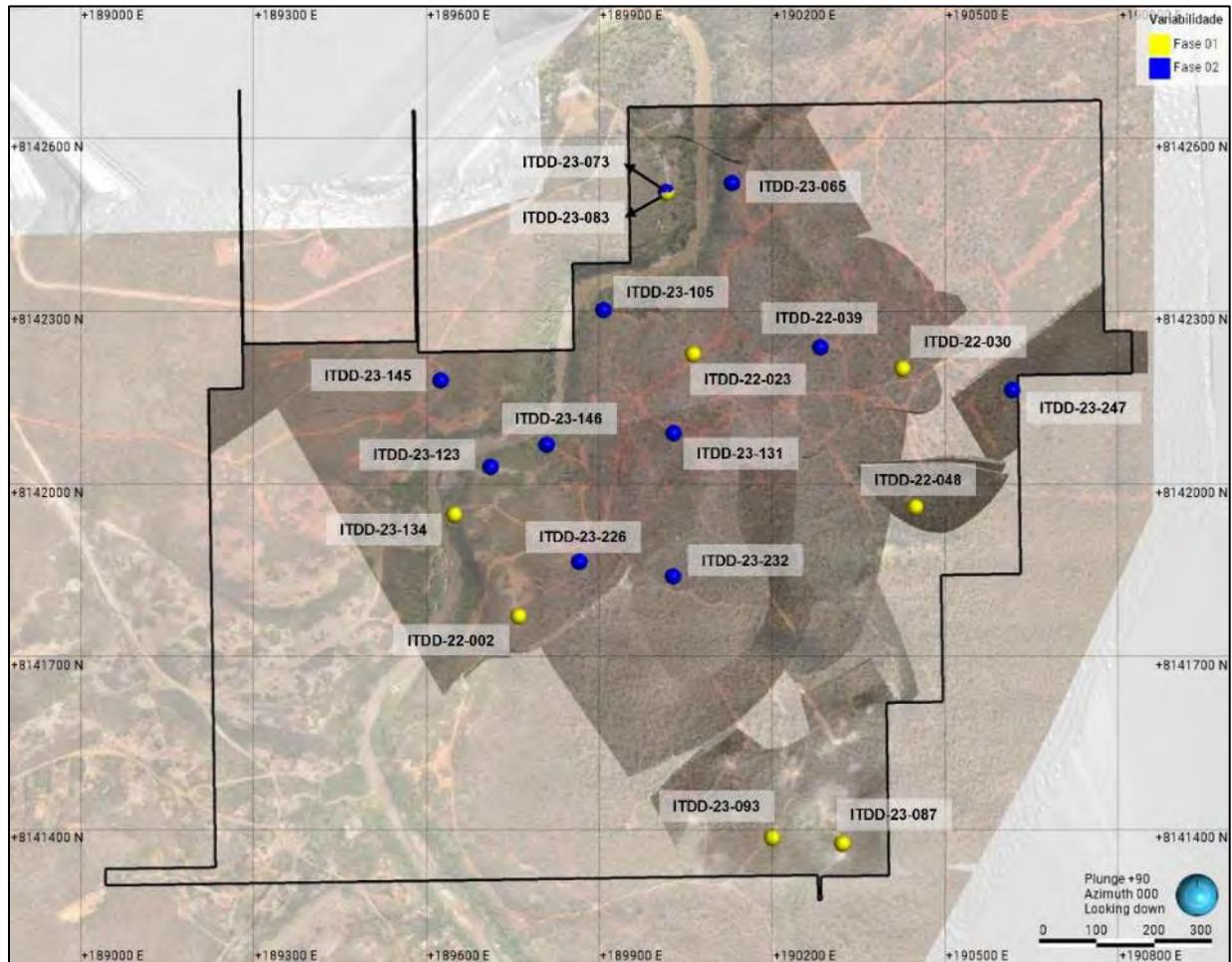
Figure 13-20: Variability Additional Drill-Hole Locations (Phase 2 in Blue)
