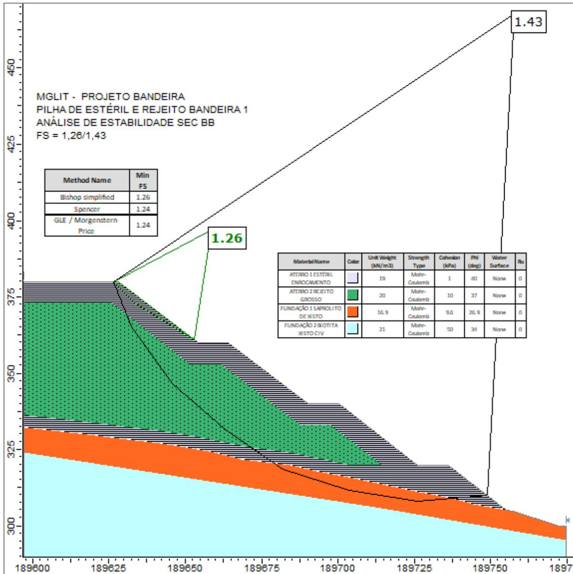
Figure 18-17: Stability Analysis of Section BB, FOS = 1.26/1.43
