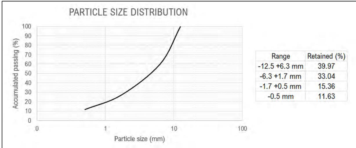
Figure 13-2: Product Size Distribution After Crushing to P<sub>100</sub> 12.7 mm
