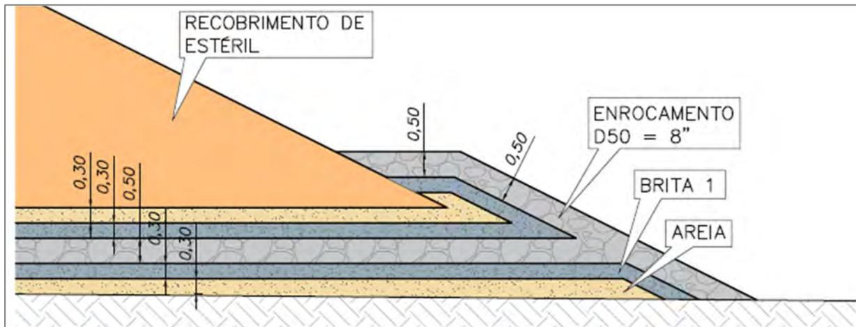
Figure 18-23: Typical Foot Drain Section
