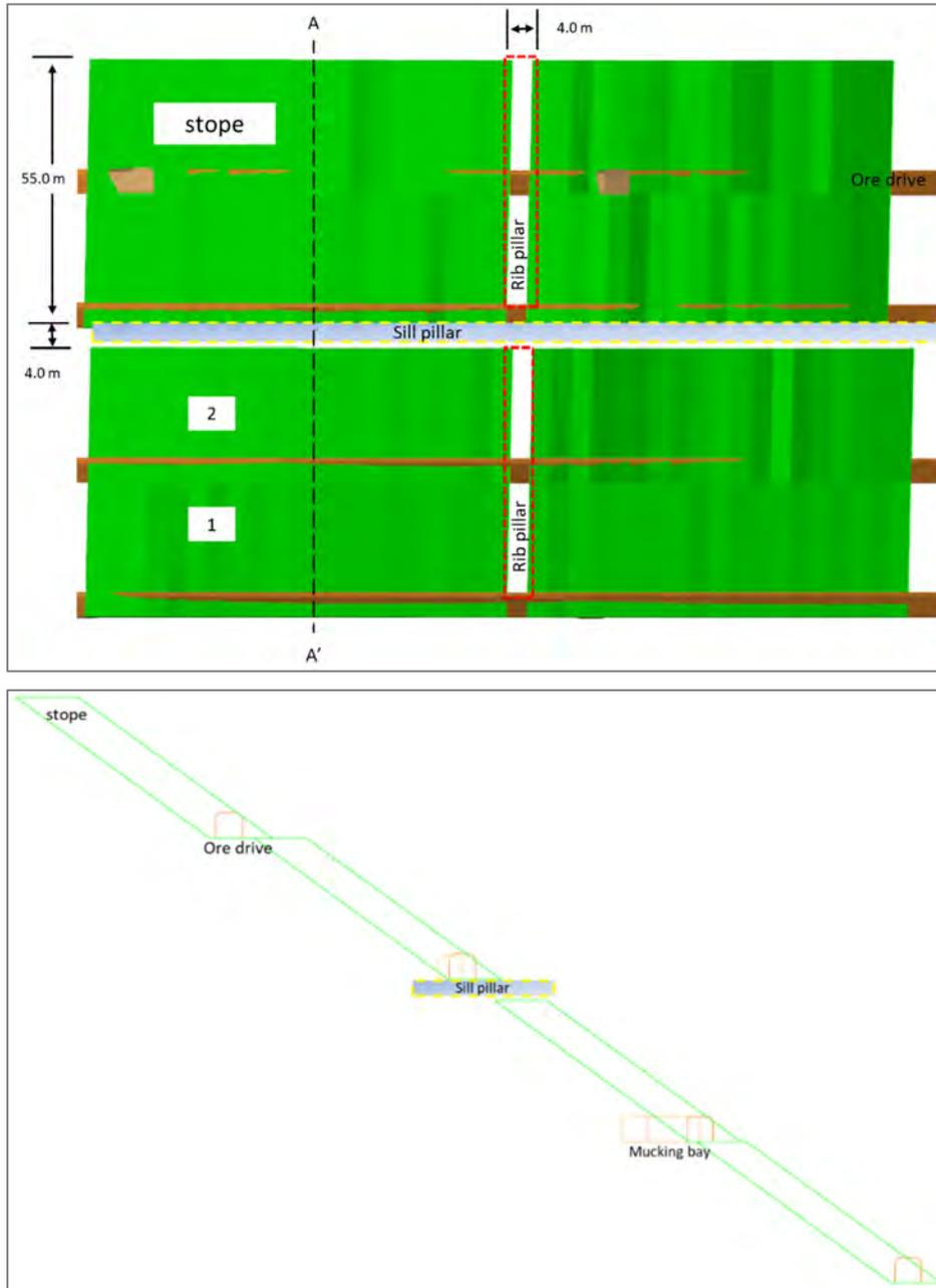
*Figure 16-9: Typical Panel of the Bandeira Mine*
