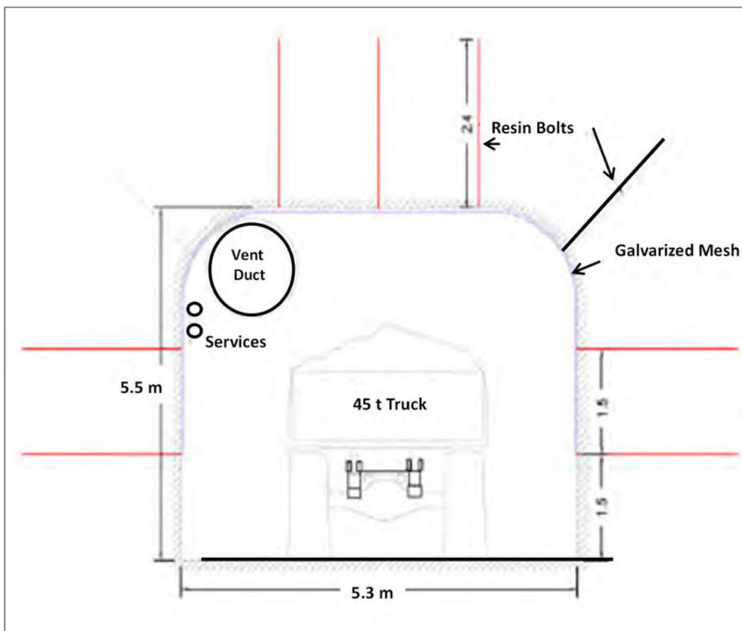
*Figure 16-7: Typical Section of the Decline*
