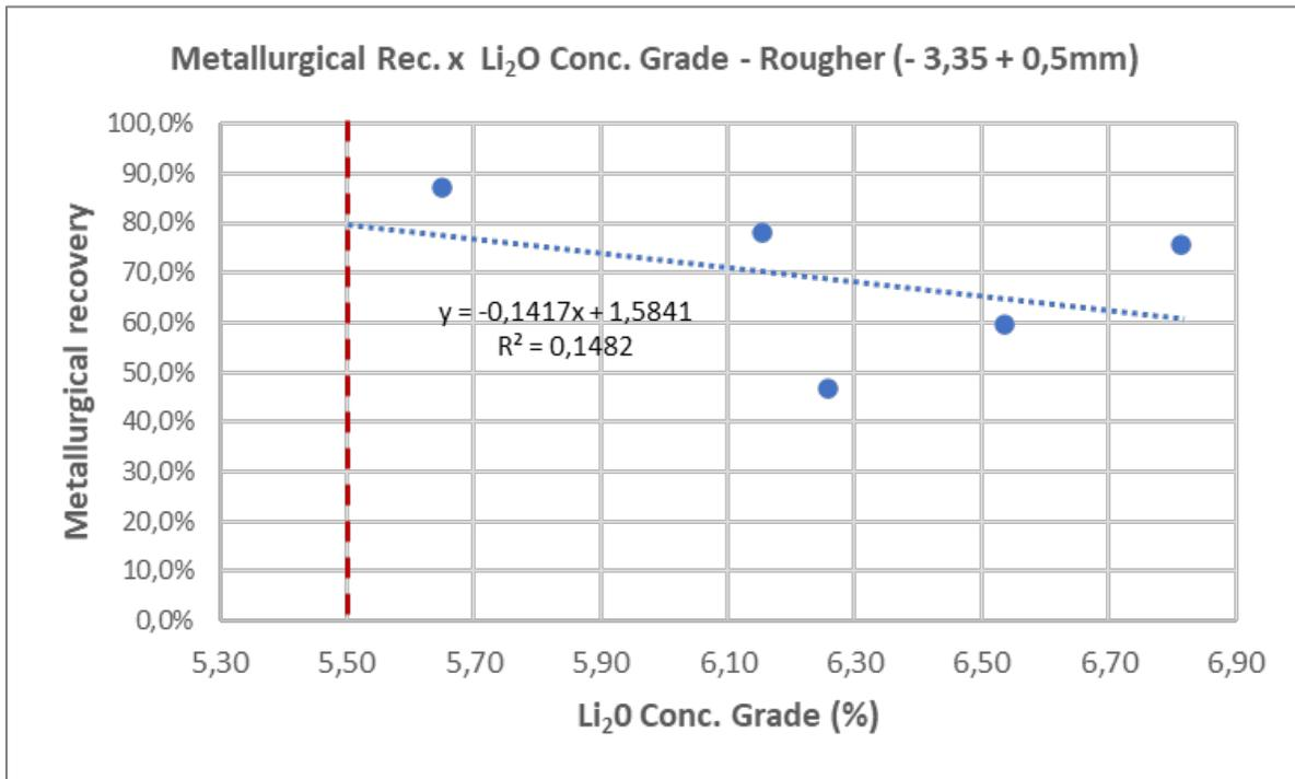
Figure 13-31: Rougher Medium Metallurgical Recovery x Li<sub>2</sub>O Grade in Concentrate
