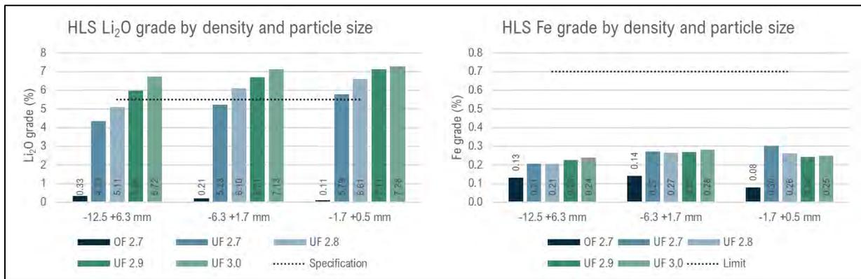
Figure 13-5: Li<sub>2</sub>O and Fe Chemical Analysis Results for each HLS Step
