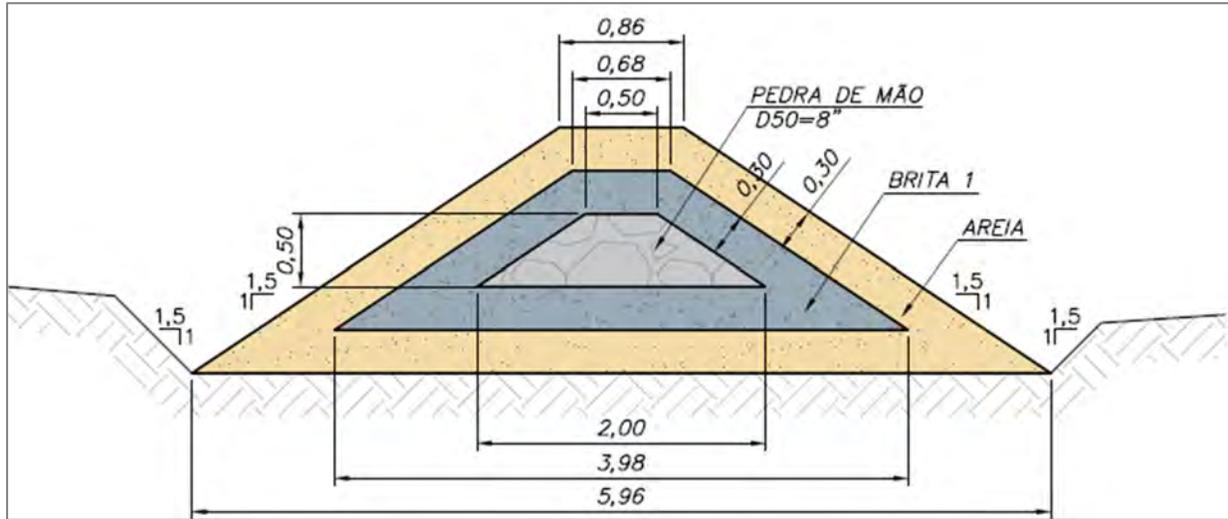
Figure 18-22: Typical Bottom Drain Device Cross Section
