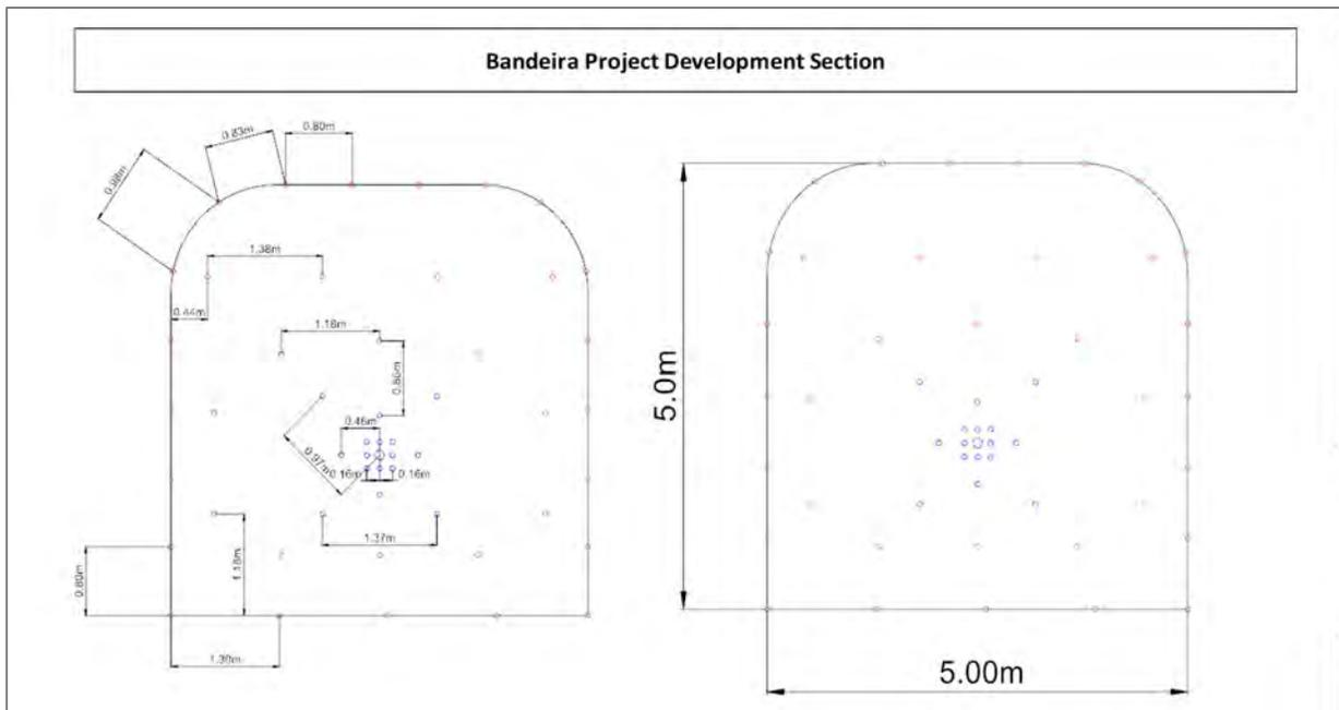
Figure 16-25: Drilling and Blasting Plan for the Drives
