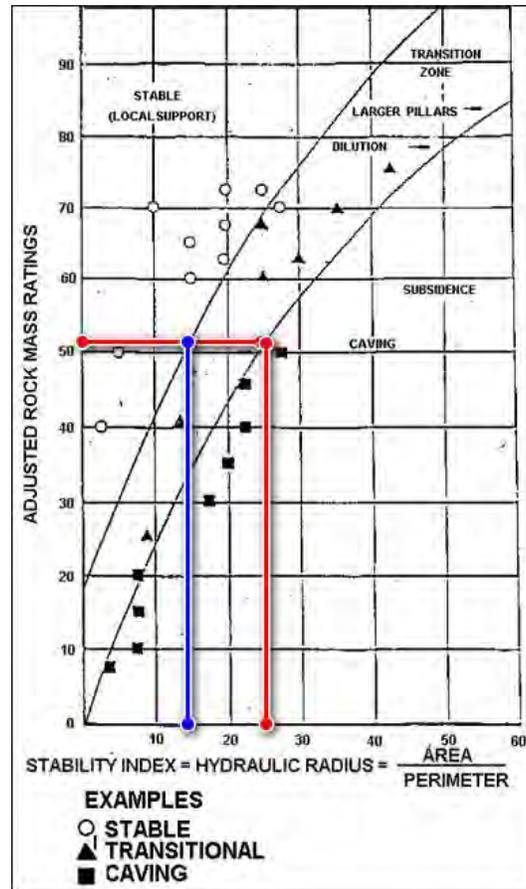
Figure 16-3: Correlation Between MRMR and Stability Index for an MRMR Value of 51.77
