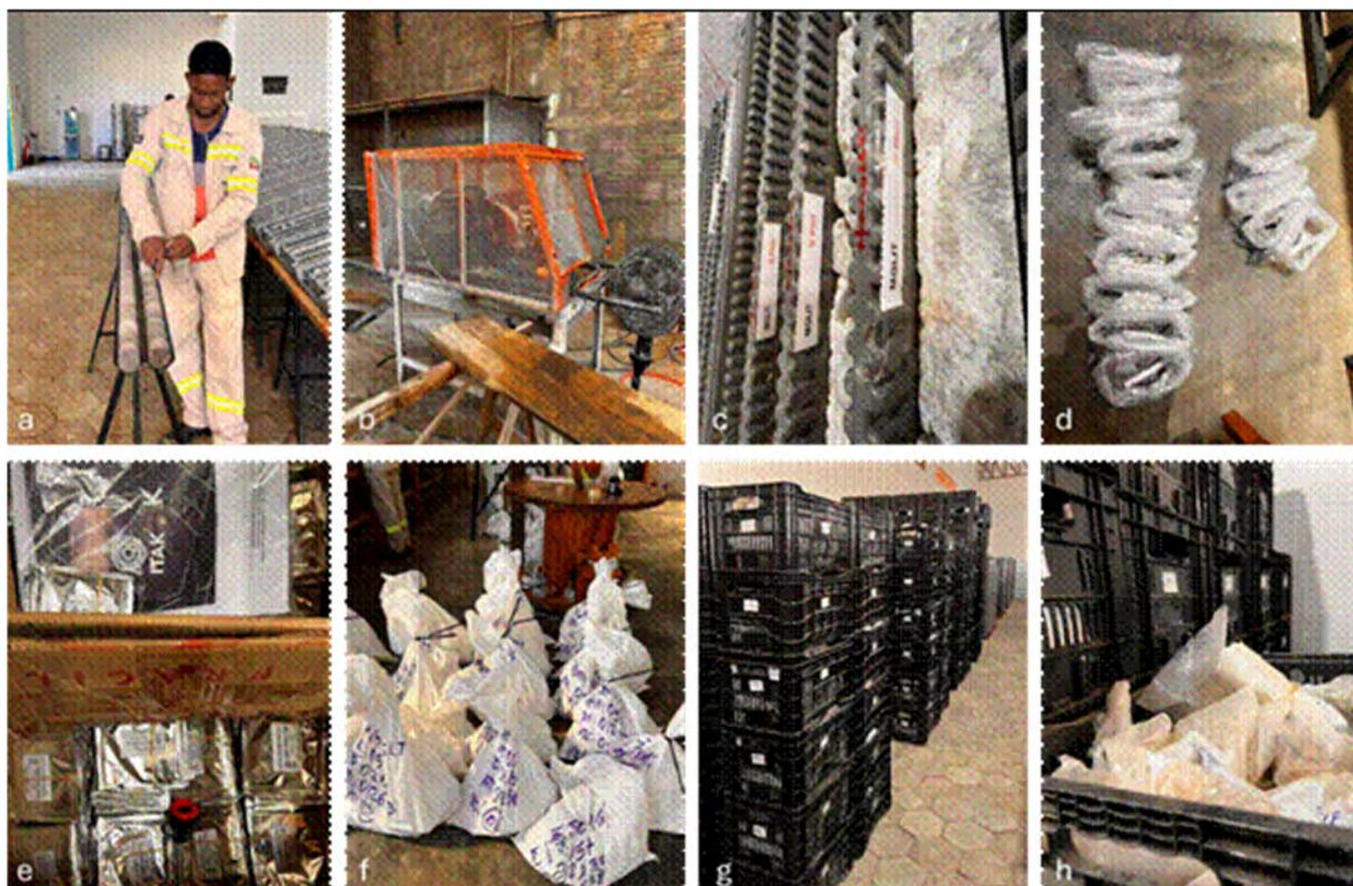
Notes: a) Marking for Sawing; b) Core saw; c) Cores after Sampling with Assays Identified; d) Identified Samples to Send to Lab; e) QA/QC—Standard to Insert in Batch; f) Batch to Send to Lab; g and h) Storage of Pulverized Samples and Crushed Samples after Return from Labs, Custody Chair.
