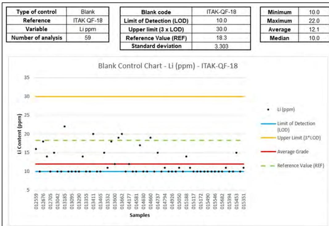
Figure 11-5: Blank Control Chart—ITAK QF-18
