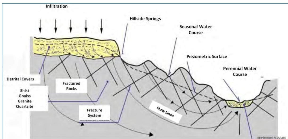
*Figure 16-5: Conceptual Model of Regional Groundwater Circulation*
