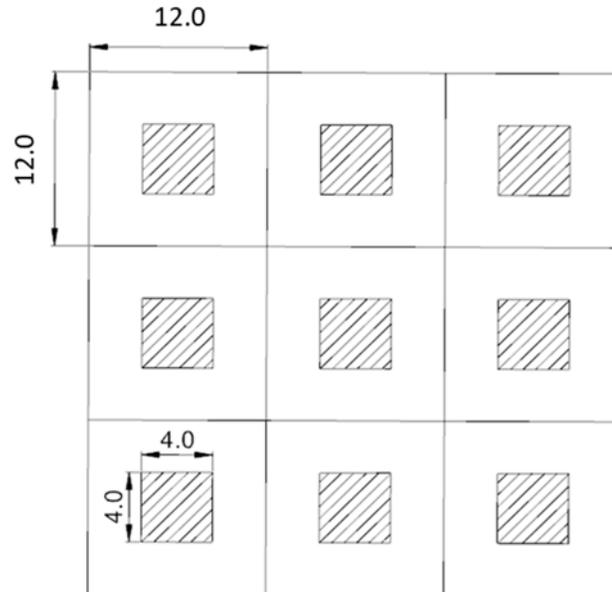
Figure 16-10: Schematic Drawing of the Room-and-Pillar Mining Method
