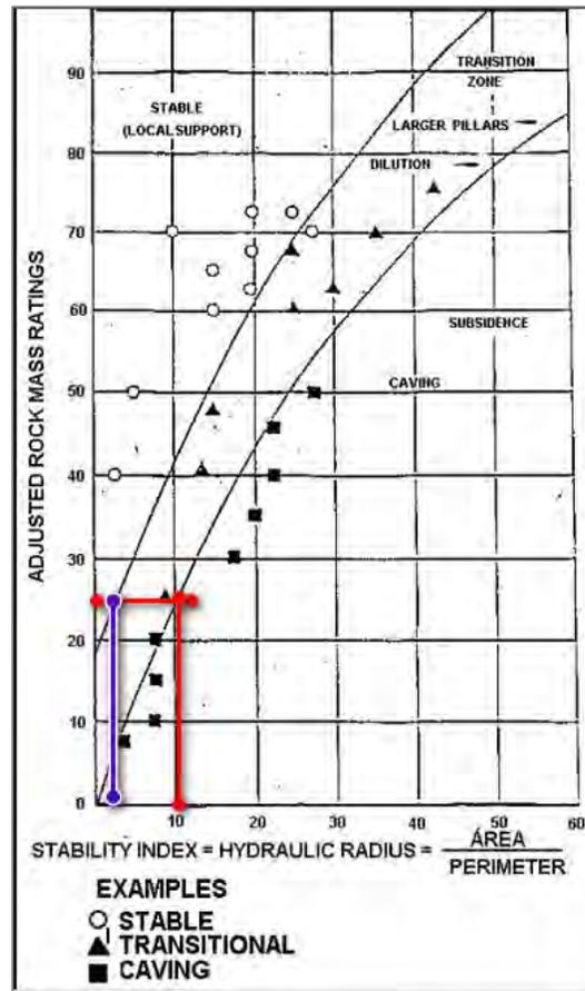
Figure 16-2: Correlation Between MRMR And Stability Index for an MRMR Value of 23.68
