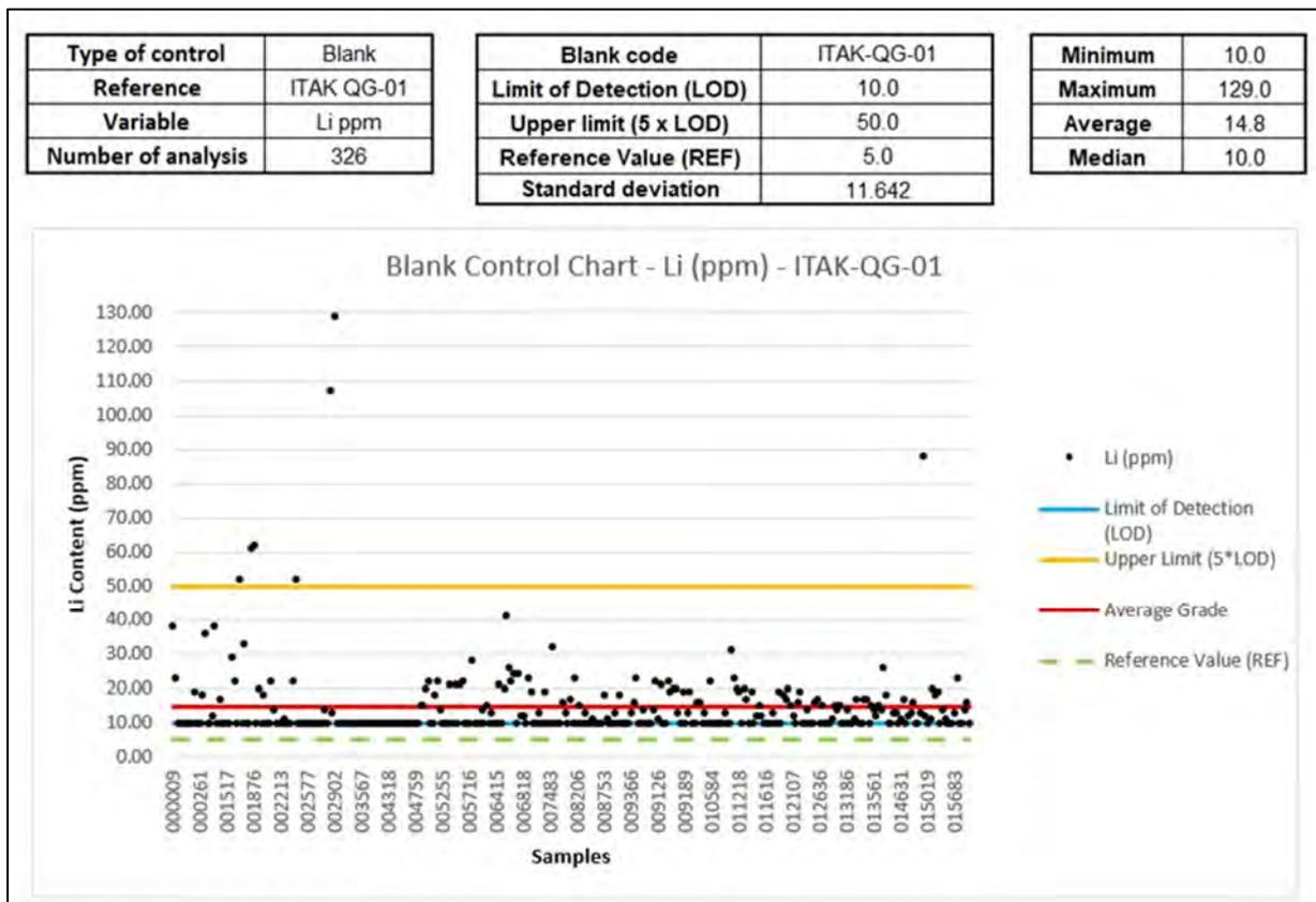
Figure 11-2: Blank Control Chart—ITAK QG-01
