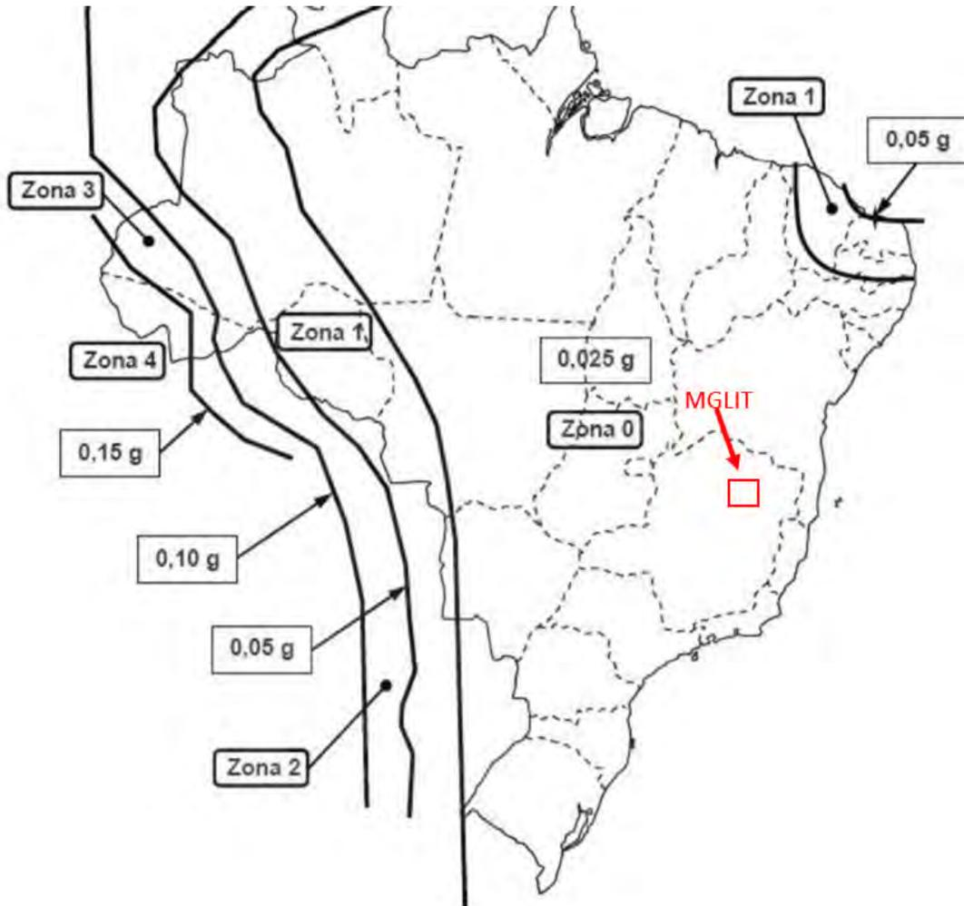
Figure 18-11: Seismic Zones of NBR 15421
