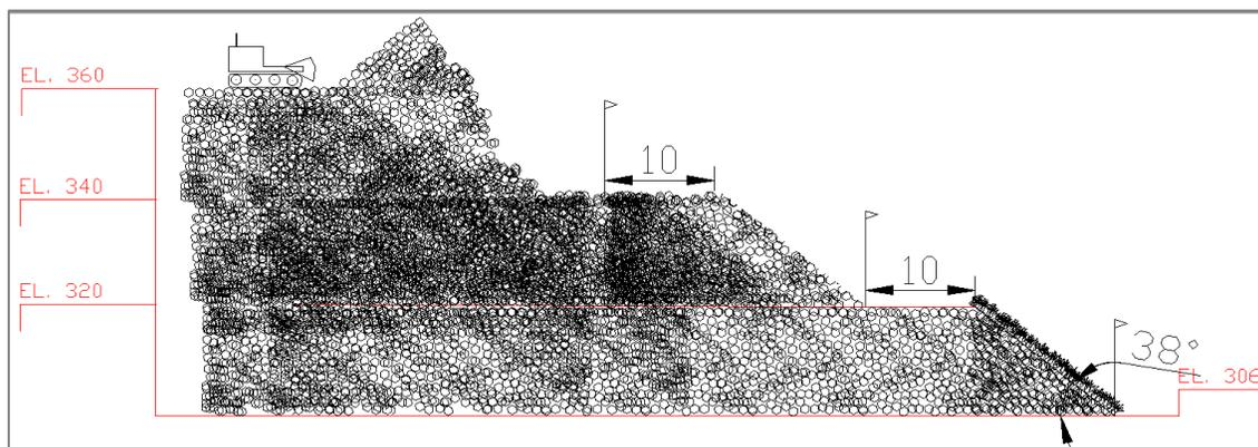
*Figure 18-16: Construction Sequence of the Benches. Once the Position of the Berm Is Reached, Mark the Next Berm Again, Until the Dump is Complete*
