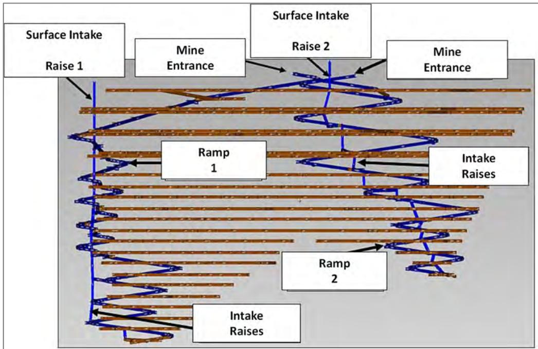
Figure 16-26: Schematic Air Intake Circuit for the Mine
