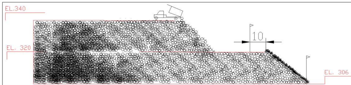
*Figure 18-15: Reached at El. 320 m Mark A Line of Flags 10 m from the Crest, which will be the Edge of Bank 320*
