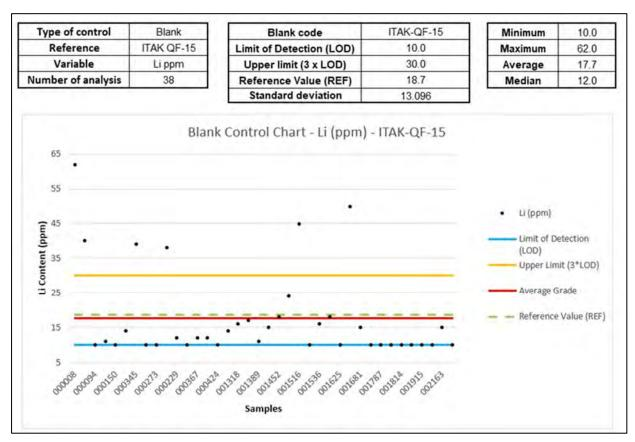
Figure 11-3: Blank Control Chart—ITAK QF-15
