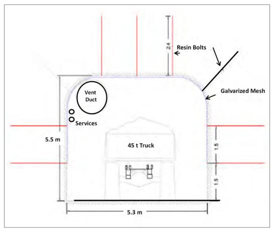
Figure 16-7: Typical Section of the Decline
