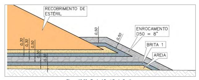
Figure 18-23: Typical Foot Drain Section
