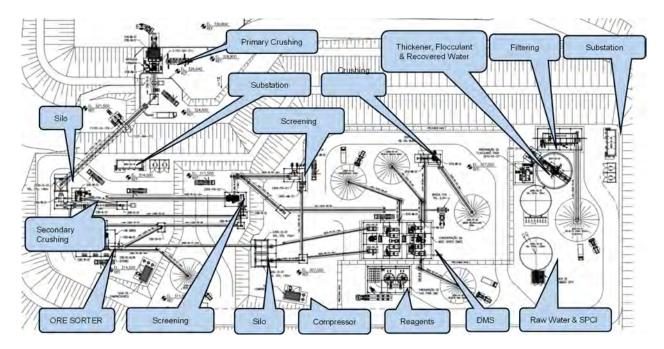
Figure 18-6: General Layout of the Processing Plant
