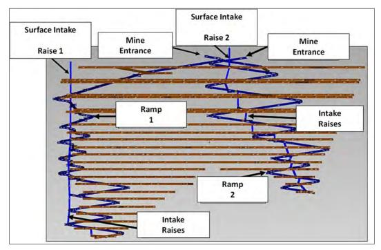
Figure 16-26: Schematic Air Intake Circuit for the Mine
