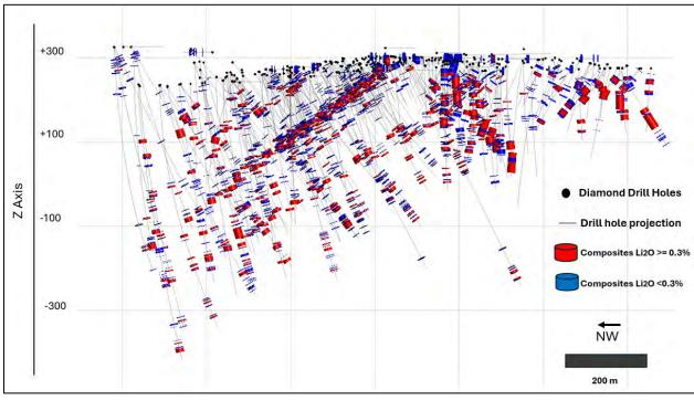
Figure 14-2: Assay Composites Classified by Li<sub>2</sub>O >0.3% Grade Limit in Pegmatites Veins (Oblique View NW−SE)
