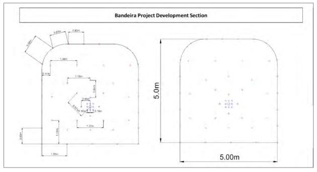
Figure 16-25: Drilling and Blasting Plan for the Drives
