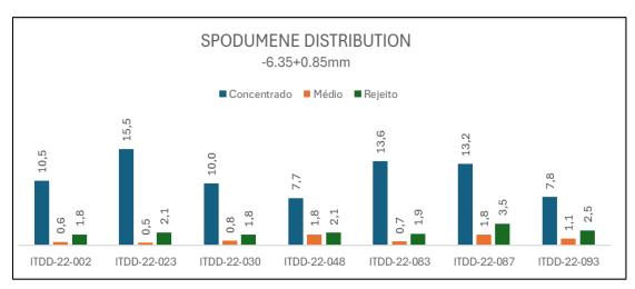
Figure 13-13: Spodumene Mass Distribution in HLS Test for Fine Material (-6.35 +0.85 mm)
