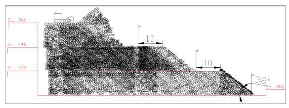
Figure 18-16: Construction Sequence of the Benches. Once the Position of the Berm Is Reached, Mark the Next Berm Again, Until the Dump is Complete
