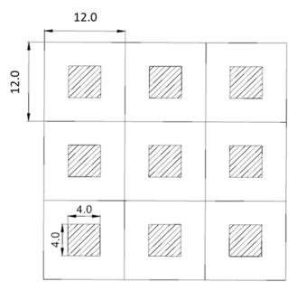
Figure 16-10: Schematic Drawing of the Room-and-Pillar Mining Method
