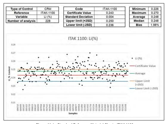
Figure 11-6: Standard Reference Material Chart—ITAK 1100
