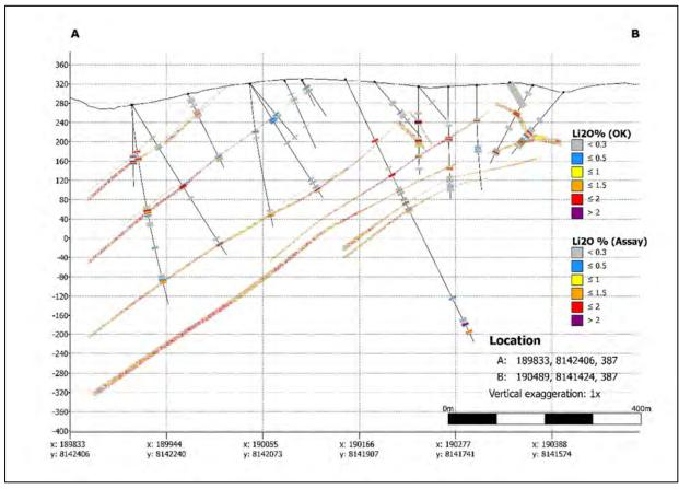
Figure 14-14: Bandeira Project Li<sub>2</sub>O % Grades Estimation (Cross-Section)
