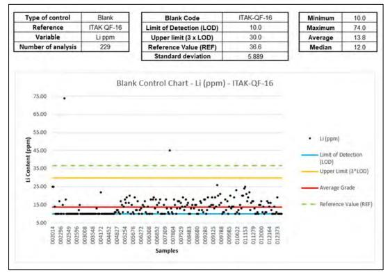
Figure 11-4: Blank Control Chart—ITAK QF-16
