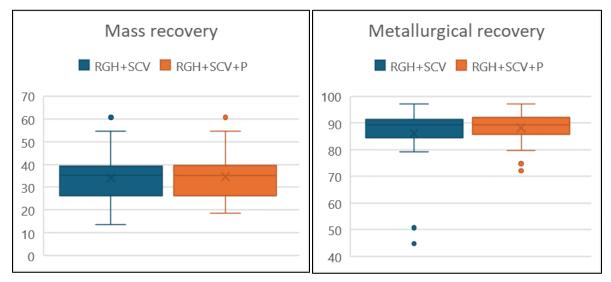
Figure 13-22: Comparative Recovery for 2-Stage and 3-Stage Circuits (-12.7 mm +0.5 mm)
