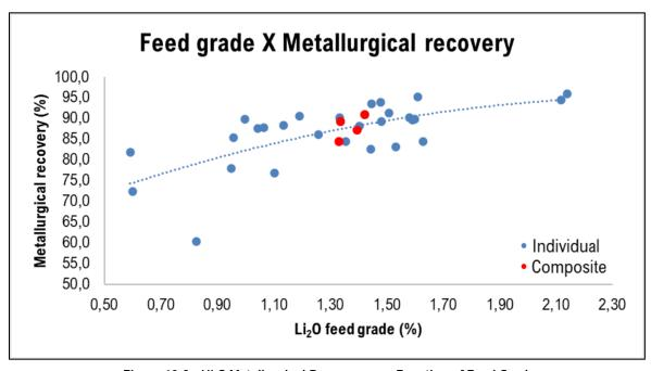
Figure 13-9: HLS Metallurgical Recovery as a Function of Feed Grade
