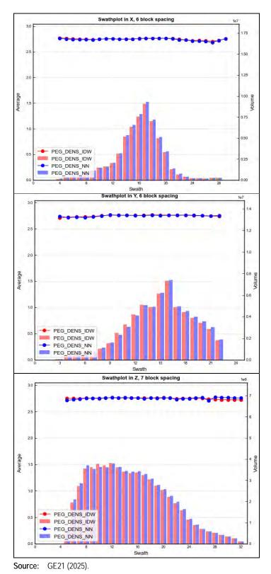
Figure 14-18: Estimation Validation—Swath Plot on the X, Y, and Z Axes for Density
