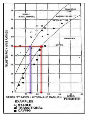
Figure 16-4: Correlation Chart Between MRMR and Stability Index for an MRMR Value of 49.62 in Pegmatite
