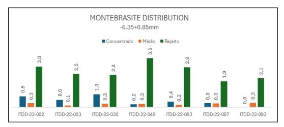
Figure 13-15: Montebrasite Mass Distribution in HLS Test for Fine Material (-6.35 +0.85 mm)
