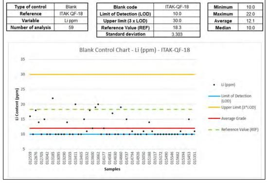
Figure 11-5: Blank Control Chart—ITAK QF-18
