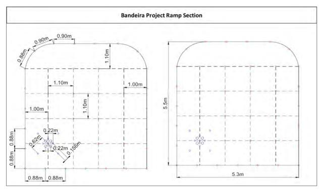
Figure 16-24: Drilling and Blasting Plan for the Ramps
