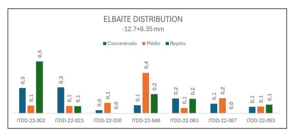
Figure 13-18: Elbaite Mass Distribution in HLS Test for Coarse Material (-12.7 +6.35 mm)
