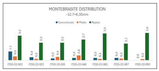
Figure 13-14: Montebrasite Mass Distribution in HLS Test for Coarse Material (-12.7 +6.35 mm)
