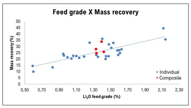
Figure 13-10: HLS Mass Recovery as a Function of Feed Grade
