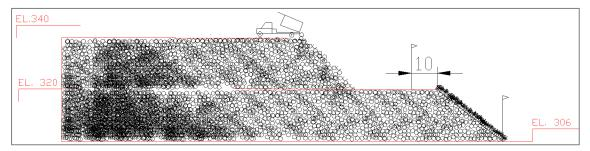
Figure 18-15: Reached at El. 320 m Mark A Line of Flags 10 m from the Crest, which will be the Edge of Bank 320
