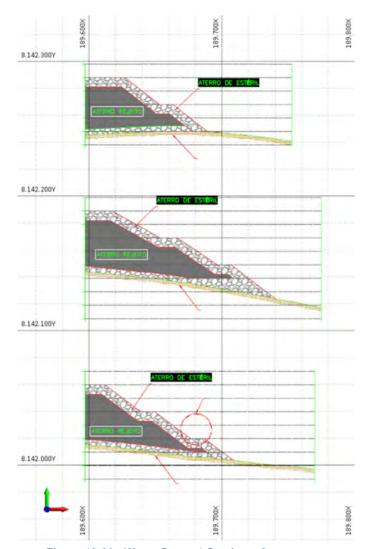
Figure 18-20: Waste Dump 1 Section—Arrangement
