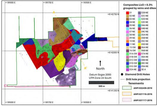
Figure 14-4: Spodumene Grade Shells Modelled with Assay Composites Li<sub>2</sub>O >0.3% (Plan View)
