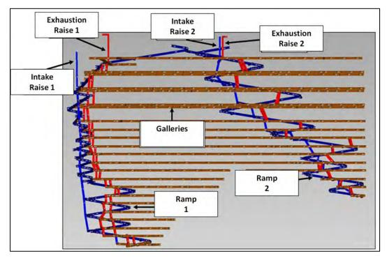
Figure 16-28: Schematic Main Mine Ventilation System
