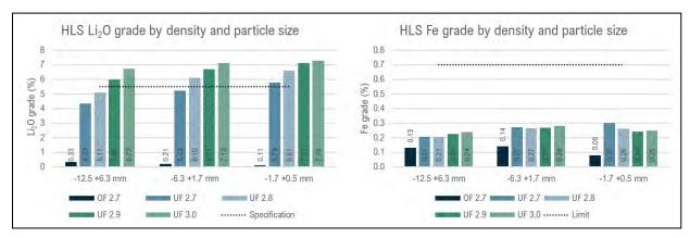
Figure 13-5: Li<sub>2</sub>O and Fe Chemical Analysis Results for each HLS Step
