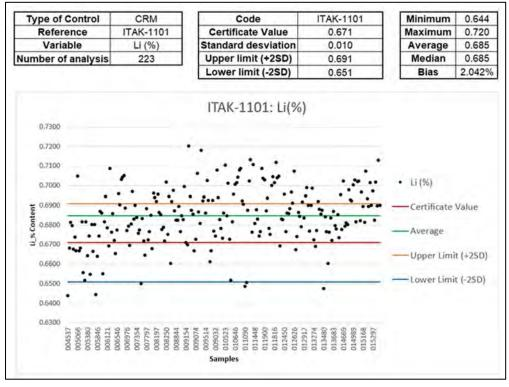
Figure 11-7: Standard Reference Material Chart—ITAK 1101
