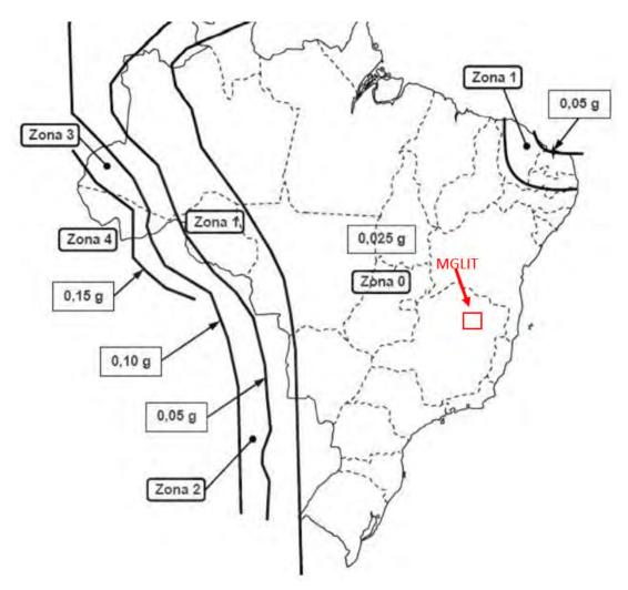
Figure 18-11: Seismic Zones of NBR 15421
