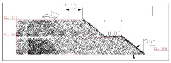
Figure 18-14: Geometries for the Formation of the Bank Edge
