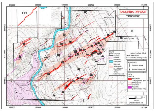
Figure 9-3: Bandeira Deposit Trench Sample Map—22 Trenches Sited Preferentially in Soil Anomalies, Most of Which Intercepted Pegmatites
