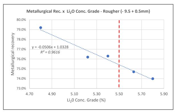
Figure 13-32: Rougher Composite Metallurgical Recovery x Li<sub>2</sub>O Grade in Concentrate
