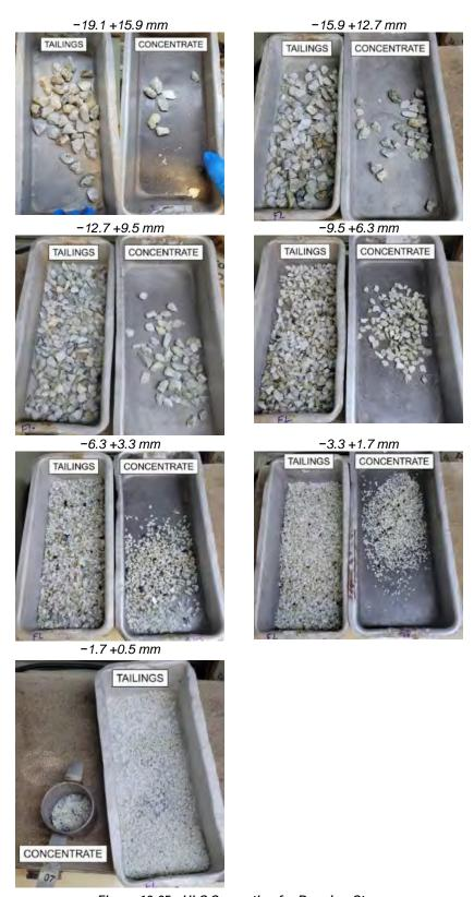
Figure 13-25: HLS Separation for Rougher Stage
