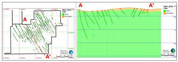
Figure 14-6: Weathering Zone Model (Left, Plan View; Right, Cross-Section View)
