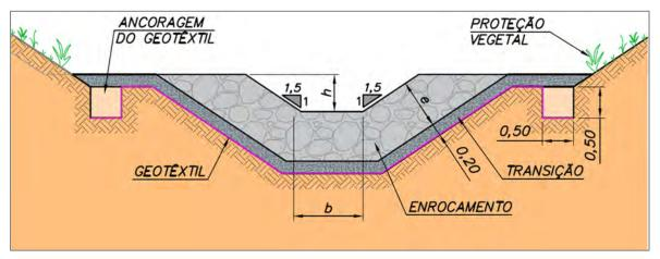
Figure 18-19: Typical Section of Hydraulic Devices Consisting of a Trapezoidal Channel with Rockfill Lining
