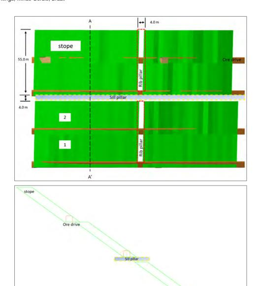
Figure 16-9: Typical Panel of the Bandeira Mine
