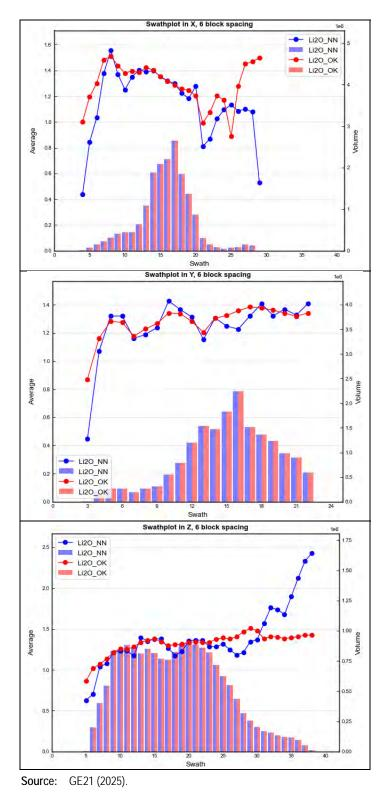
Figure 14-17: Estimation Validation—Swath Plot on the X, Y, and Z Axes for Li<sub>2</sub>O Grades
