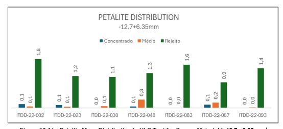
Figure 13-16: Petalite Mass Distribution in HLS Test for Coarse Material (-12.7 +6.35 mm)
