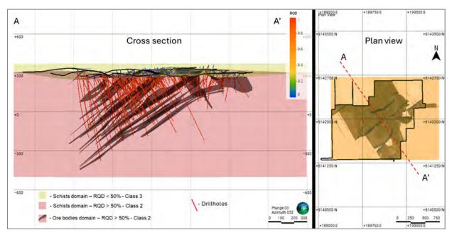
Figure 16-1: Bandeira Project Geotechnical Domains—Left, Cross-Section View; Right, Plan View
