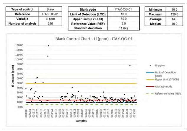
Figure 11-2: Blank Control Chart—ITAK QG-01
