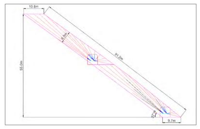
Figure 16-23:Longhole Drilling
