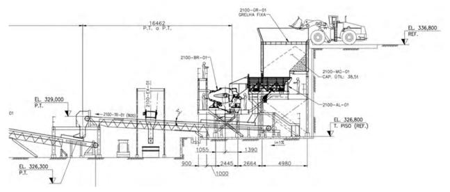
Figure 17-3: Primary Crushing
