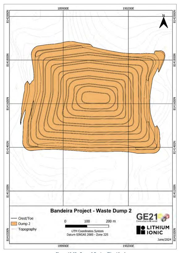
Figure 18-25: Dump 2 Design (Plan View)
