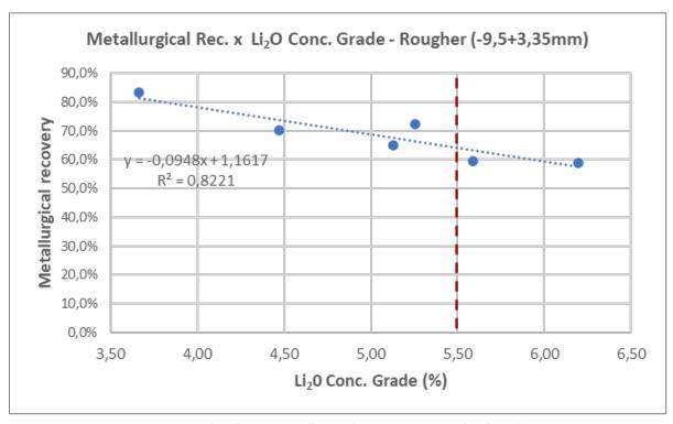
Figure 13-30: Rougher Coarse Metallurgical Recovery x Li<sub>2</sub>O Grade in Concentrate
