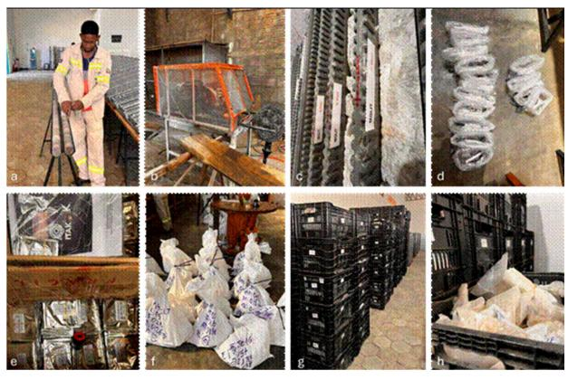
a) Marking for Sawing; b) Core saw; c) Cores after Sampling with Assays Identified; d) Identified Samples to Send to Lab; e) QA/QC—Standard to Insert in Batch; f) Batch to Send to Lab; g and h) Storage of Pulverized Samples and Crushed Samples after Return from Labs, Custody Chair. Notes:
