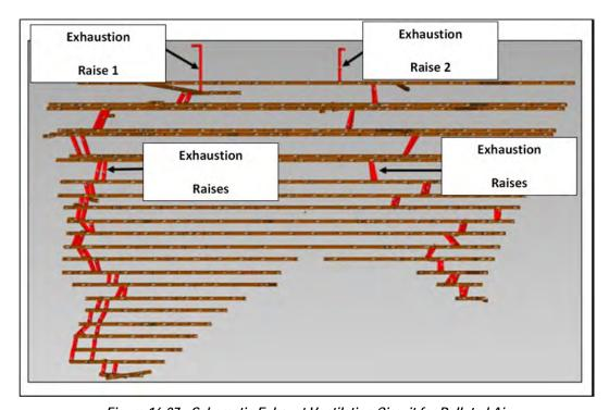
Figure 16-27: Schematic Exhaust Ventilation Circuit for Polluted Air
