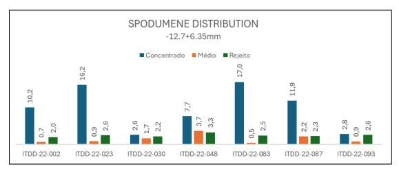
Figure 13-12: Spodumene Mass Distribution in HLS Test for Coarse Material (-12.7 +6.35 mm)
