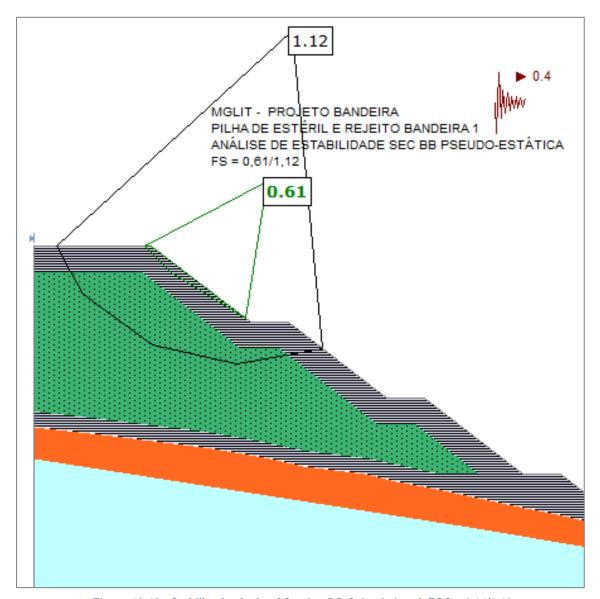
Figure 18-18: Stability Analysis of Section BB Seismic Load, FOS = 0.61/1.12
