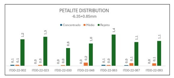
Figure 13-17: Petalite Mass Distribution in HLS TEST for Fine Material (-6.35 +0.85 mm)
