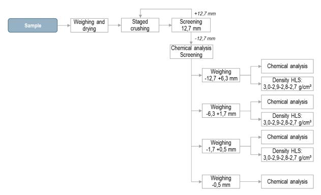
Figure 13-1: Bandeira Composite Sample Preparation Procedure
