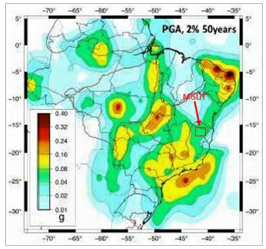
**Note:** Peak Ground Acceleration (PGA) in rock, for probabilities of 2% exceedance in 50 years, to a period of 2,475 years. **Source:** Assumpção et al. (2016).
