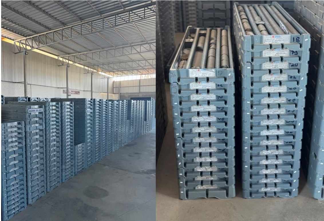
Figure 12-2: Drill core box and physical copies of all the drill hole information
