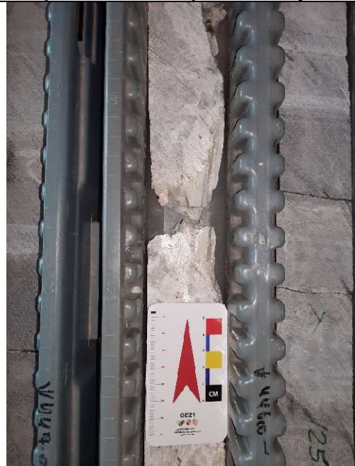
Core boxes of the modelled mineralized spodumene zone – ITDD-23-159 – 446m depth - detail of the Spodumene crystal
