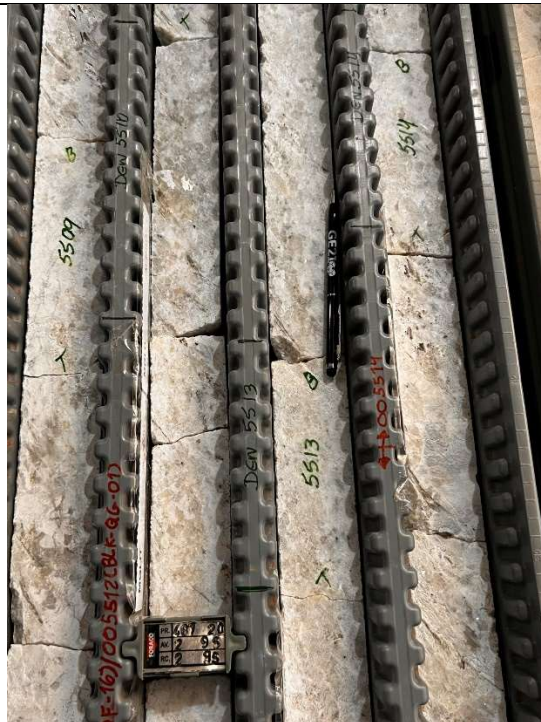
Core boxes of the modelled mineralized spodumene zone – ITDD-23-091 – 479m to 489m - samples identification
