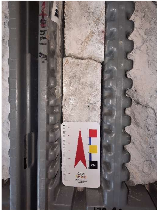
Core boxes of the modelled mineralized spodumene zone – ITDD-23-236 – – 174m depth, detail of the Spodumene crystal
