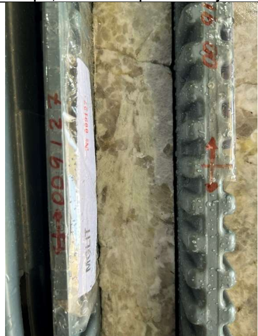
Core boxes of the modelled mineralized spodumene zone – ITDD-23-162 – 460,5m depth - detail of the Spodumene crystal
