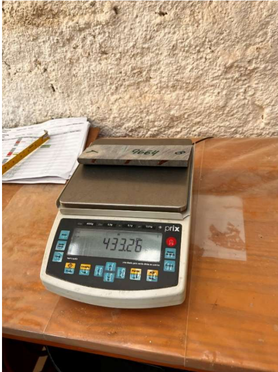
Density measurement – dry core weight
