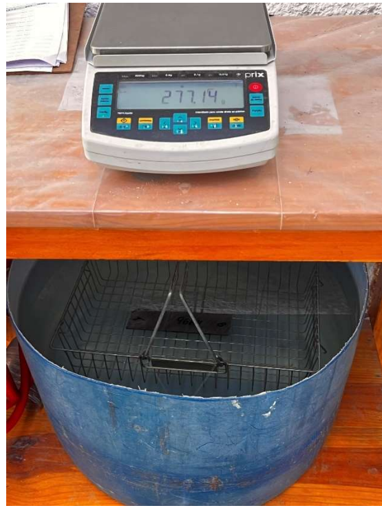
Density measurement – core weight underwater
