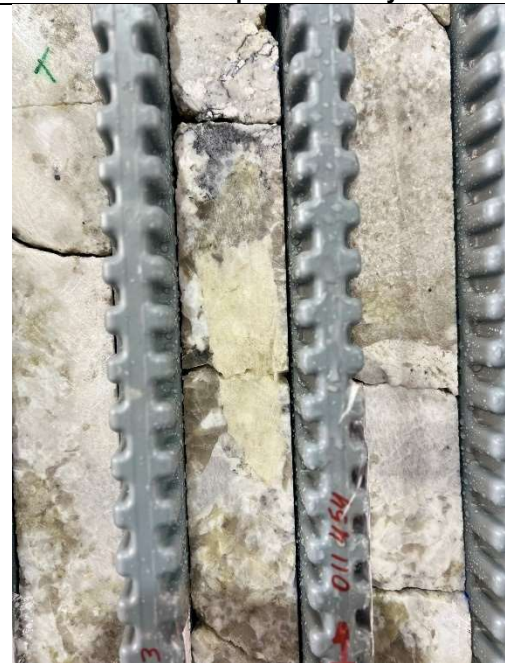
Core boxes of the modelled mineralized spodumene zone – ITDD-23-163 – 146m depth, detail of the Spodumene crystal
