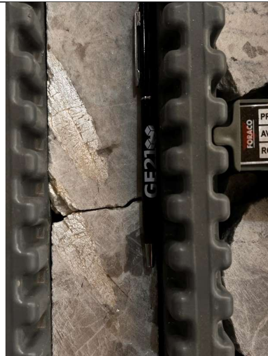
Core boxes of the modelled mineralized spodumene zone – ITDD-23-120 – 111m depth, detail of the Spodumene crystal
