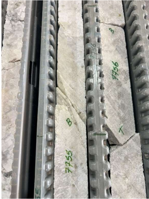
Core boxes of the modelled mineralized spodumene zone – ITDD-23-147 – – 207,80m depth, detail of the Spodumene crystal
