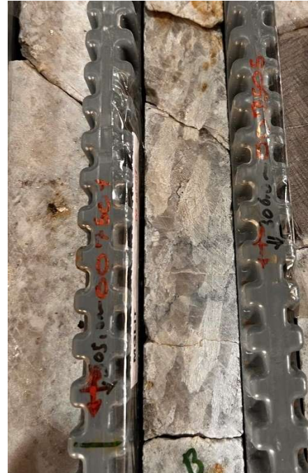
Core boxes of the modelled mineralized spodumene zone – ITDD-23-139 – 305m depth, detail of the Spodumene crystal
