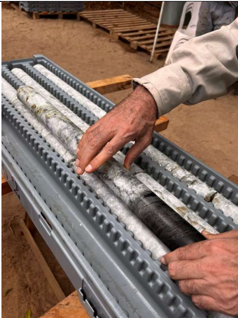
Drill Rig on site of the Bandeira, drilling in 13/09/2023 - DDH ITDD-23-192 – Spodumene in pegmatite veins cores recovered from drilling – depth 355m
